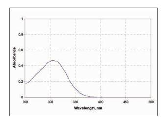
Uvinul 3039 exhibits high absorbance in the 280-320 nm region and no absorbance in the visible region (>400 nm) of the spectrum. The absorption maximum is at 306 nm in chloroform solution.
