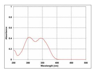
Tinuvin PA 328 exhibits high absorbance in the 300-400 nm region and minimal absorbance in the visible region (> 400 nm) of the spectrum. The absorption maxima are at 306 nm and 347 nm ( $\varepsilon$  =14760 l/mol·cm) in chloroform solution.
