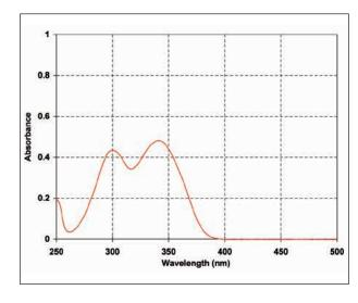
Tinuvin 329 exhibits strong absorbance in the 300-400 nm region and minimal absorbance in the visible region (>400 nm) of the spectrum. The absorption maxima are at 301 nm and 343 nm ( $\varepsilon = 15910 \text{ l/}$ mol·cm) in chloroform solution.
