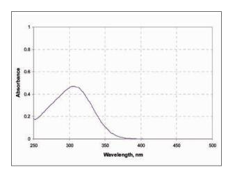
Uvinul 3035 exhibits high absorbance in the 280–320 nm region and no absorbance in the visible region (>400 nm) of the spectrum. The absorption maximum is at 307 nm in chloroform solution.
